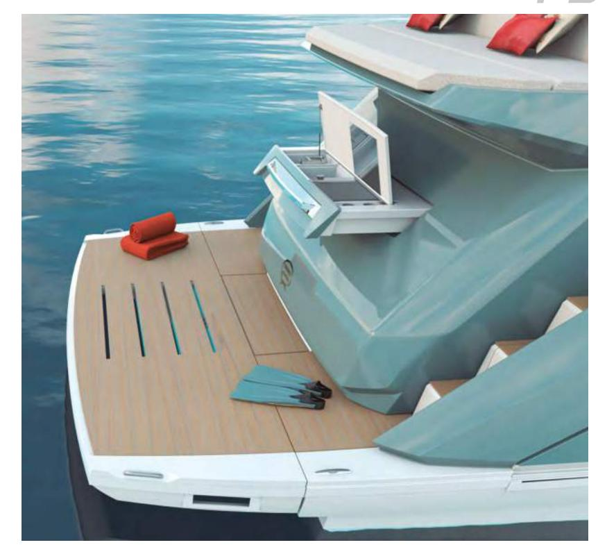
From the aft area, you can access the spacious garage, which has a hydraulic piston opening system and an electric winch, allowing for the storage of a jet ski or a tender of up to 2.80 meters, as well as extra space for accommodating water toys and diving equipment.
